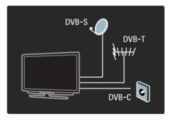
Next to the DVB-T and DVB-C reception, this TV has a built-in satellite DVB-S/S2 receiver. You can connect a satellite dish antenna and receive digital satellite channels.
